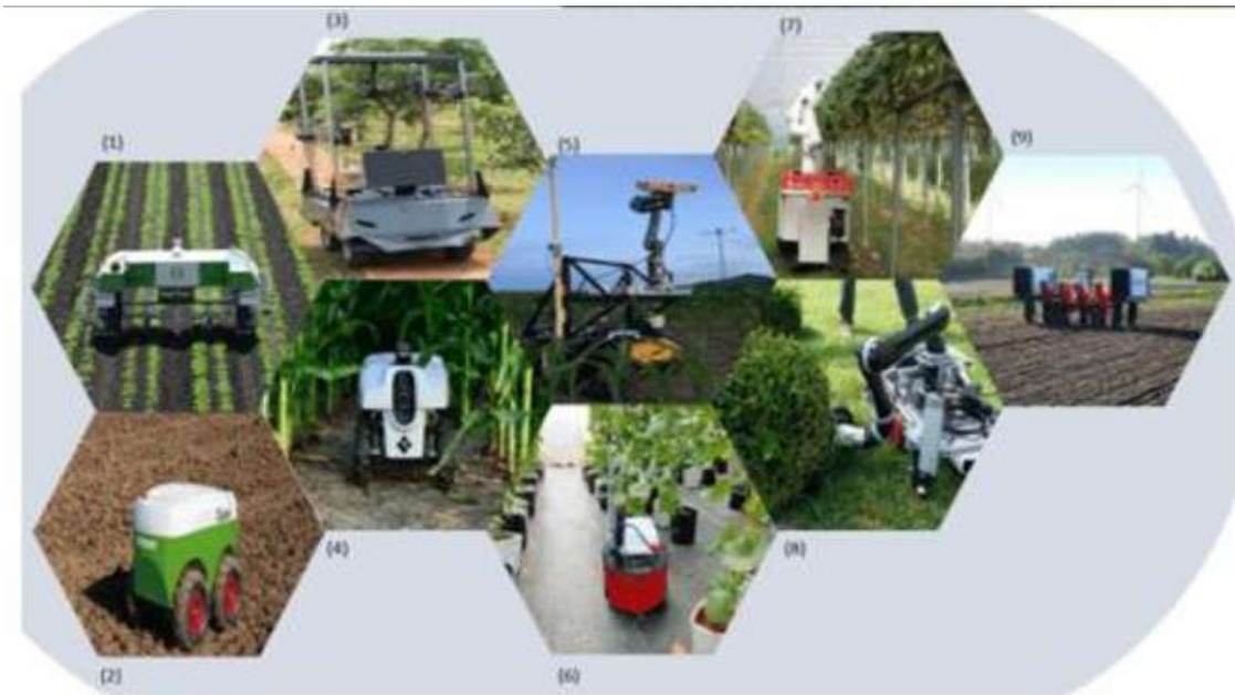
Representation of various types of agricultural robots ((1) weeding [23], (2) seeding [47], (3) disease and insect detection [55], (4) plant monitoring [69], (5) phenotyping [78], (6) spraying [86], (7) harvesting [100], (8) plant management [152], (9) multi-purpose [137]).
